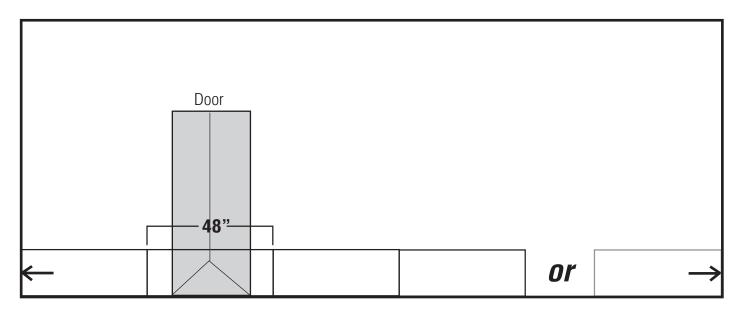
For the first course, you can start installing Strips from either gable end, or from any convenient point in the middle of the roof. You don't need to start at edge of the roof.
