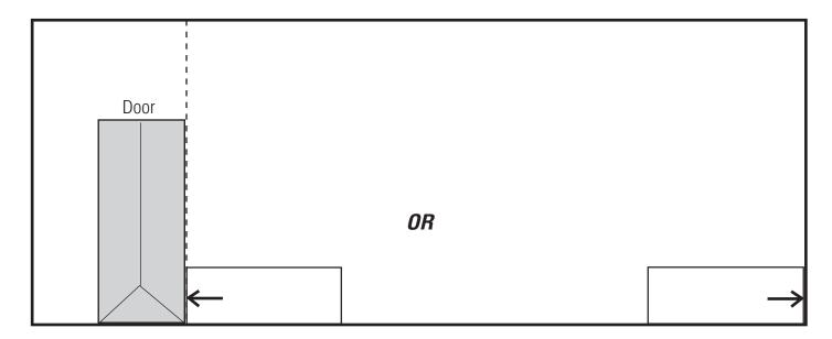
Install the fist course allowing a 1/4"gap between Shake-Strips. Its 48" from any point on one Shake-Strip to the same point on the next. Double the first course as shown. Use the guide marks to offset the joints between the top and bottom courses, just as you will for adjacent courses.
